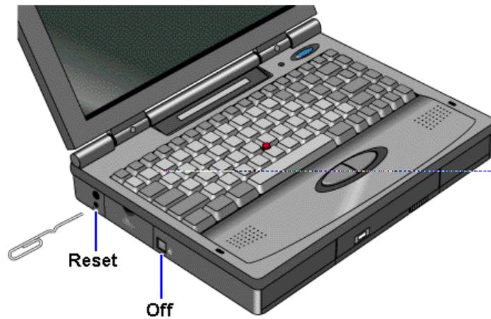
If these actions have no effect, remove the battery and ac adapter and press the reset button. Then install the battery or plug in the ac adapter and try pressing the reset button again.
