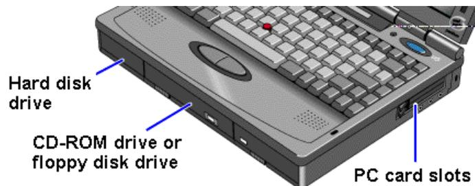
For a large hard disk drive, one that's bigger than about 2 GB (2 gigabytes, slightly more than 2 billion bytes), the hard disk may have two partitions or divisions. These two partitions appear as drive C and drive D.
