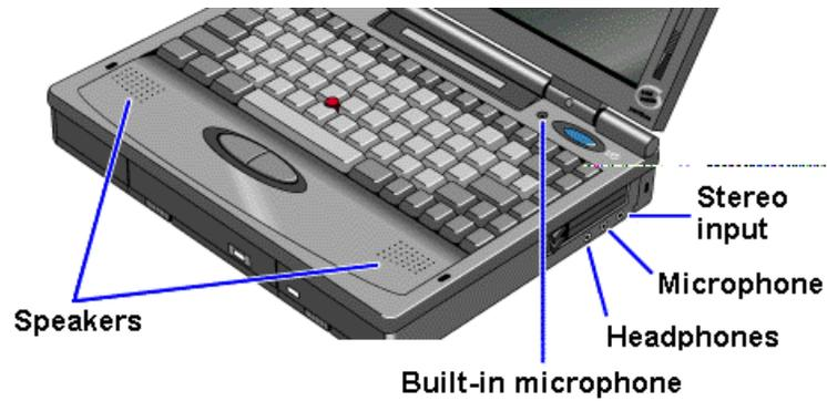
You can also plug in an external microphone, external speakers or headphones, and a stereo input source, such as a CD player.
