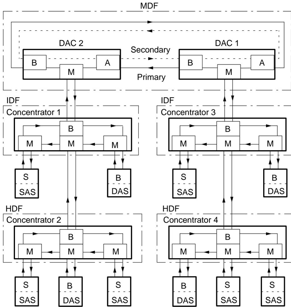
DACs1 and 2 are connected through PHY ports A and B to the dual ring.
