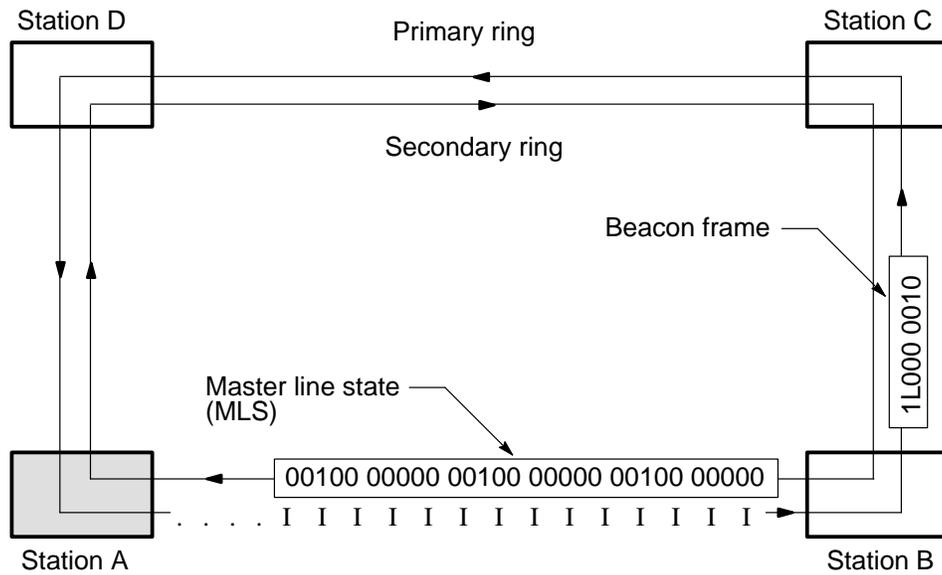
1. Defective station A transmits continuous idle symbols.
