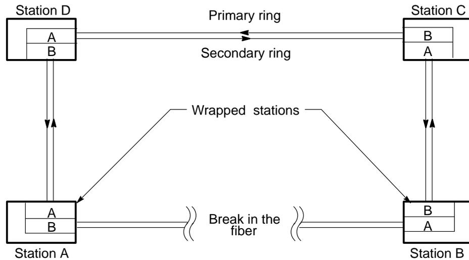
1. A break in the primary ring causes port A of station B to detect signal loss and wrap.
