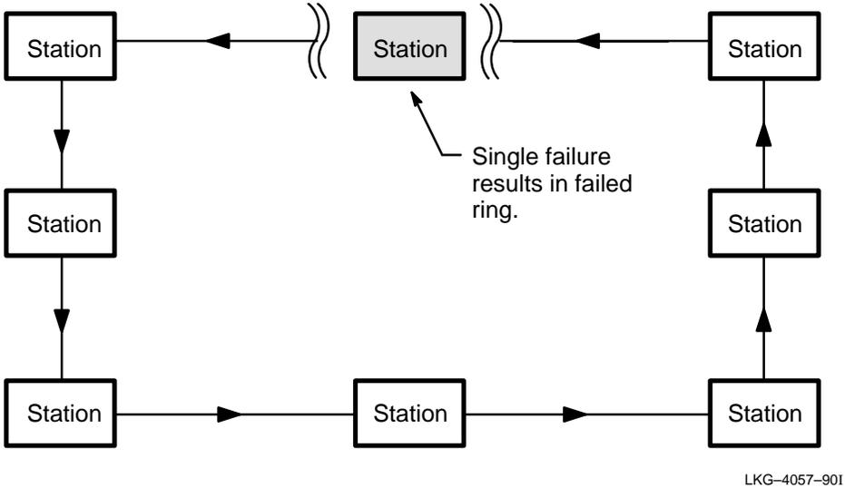
To eliminate the single-point-of-failure problem, the ANSI FDDI standards committee designed the dual ring topology. This topology solves the problem of a single failure disrupting the ring by providing a secondary transmission path. The secondary transmission path assists in start-up, initialization, and reconfiguration of the primary path.
