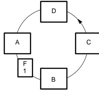
2. **A** begins transmitting the frame with Destination Address = **C** and Source Address = **A**.
