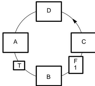
3. At completion of transmission, **A** reissues the token. **C** copies the frame addressed to it.
