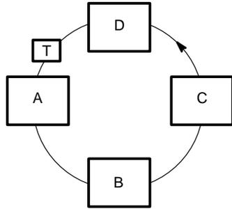
1. **A** has a frame of data to transmit and captures the token.
