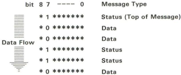
Figure 3-2. Data Flow with Status Byte Control
