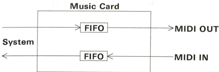
Figure 1-2. Data Flow in THRU Mode
