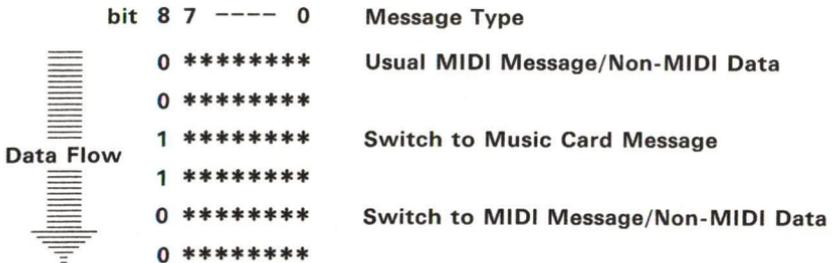
**Figure 3-1. System to MIDI Device Data Flow**
