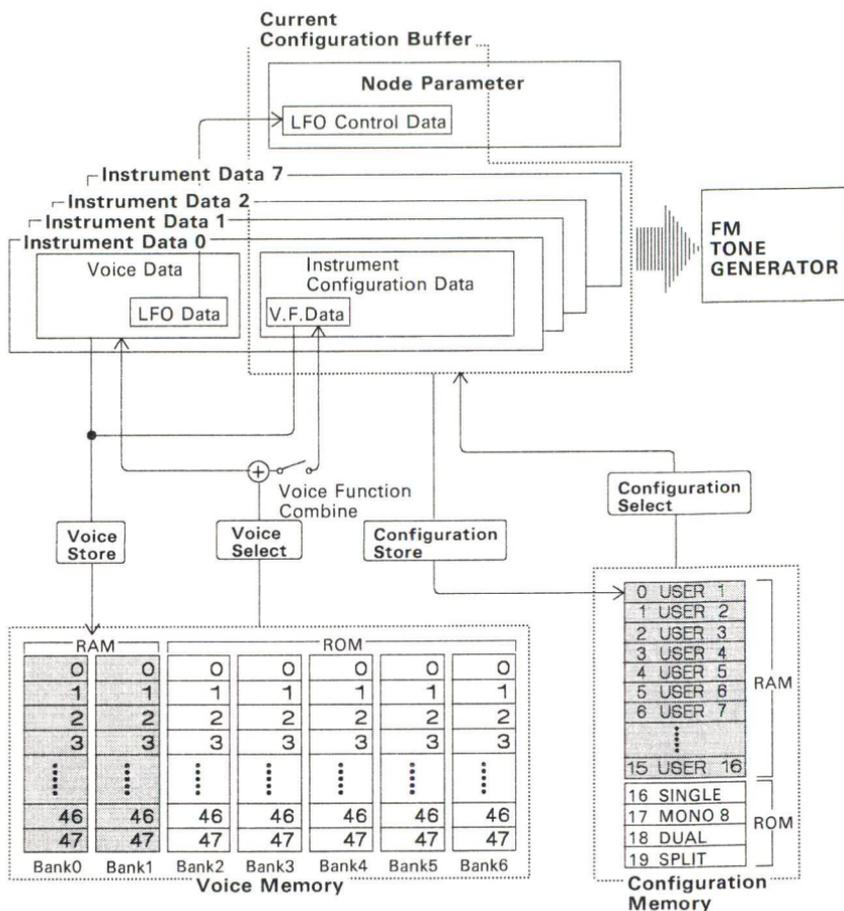
Figure 1-4. Block Diagram of the Sound Processor
