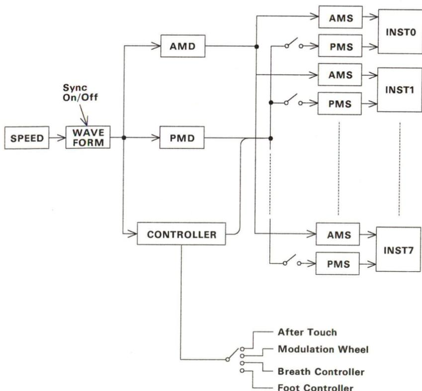
Figure 1-6. Relationship Between LFO Control Block and Instruments
