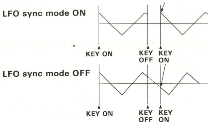
Figure 8-3. Wave Form Synchronization to KEY ON
