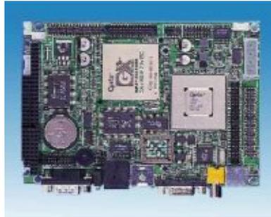
**Figure 14.16 Advantech PCM-5822 SBC**
