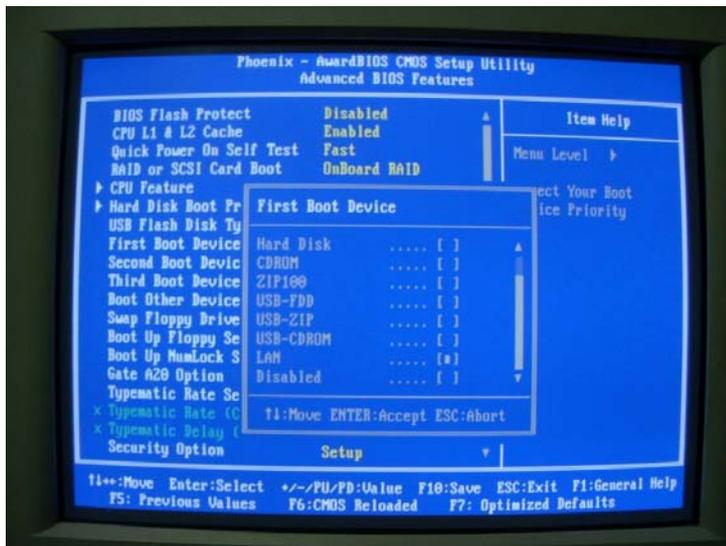
Figure 9.11 Boot from LAN in the BIOS setting
