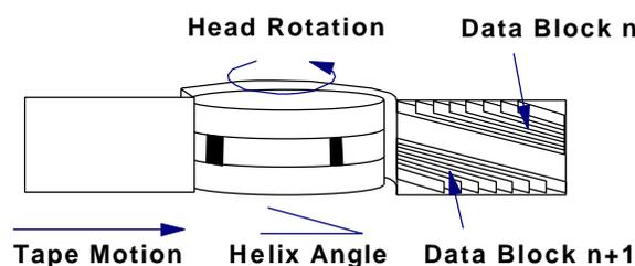
*Figure 1. Helical Scan Principles*
