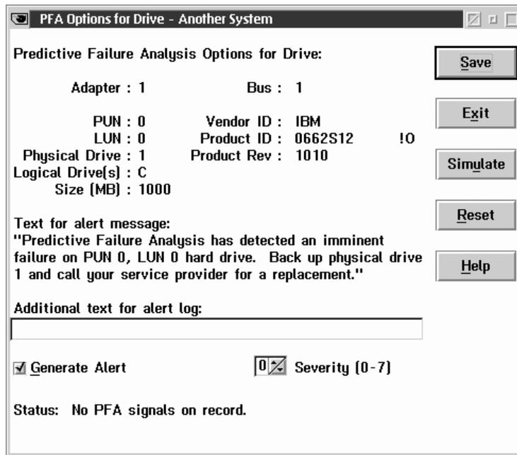
Figure 14. The PFA Options for Drive window
