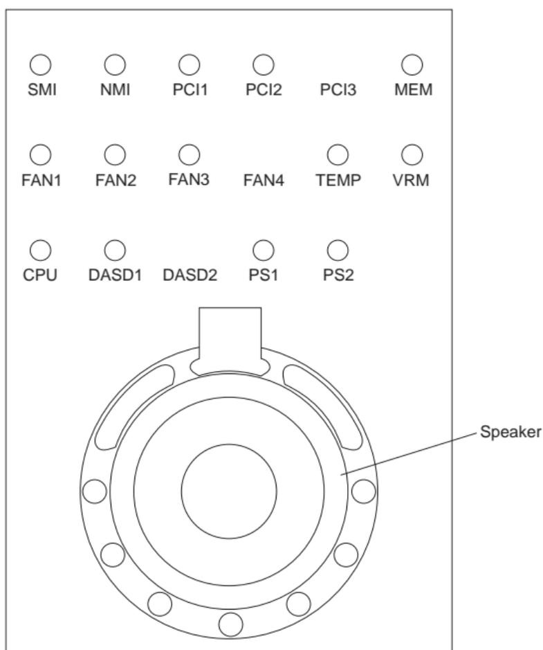
To replace the diagnostics panel LEDs, you must replace the interior LED and speaker assembly, see “Interior LED and Speaker Assembly” on page 196.
