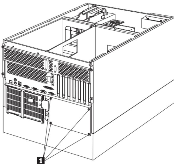
1. Remove the power supply filler plate screws **1**, then; remove the power supply filler plate.
