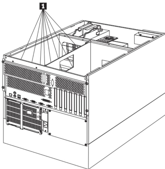
4. Remove the processor board screws **1**, then; lift the processor board out of the tray.
