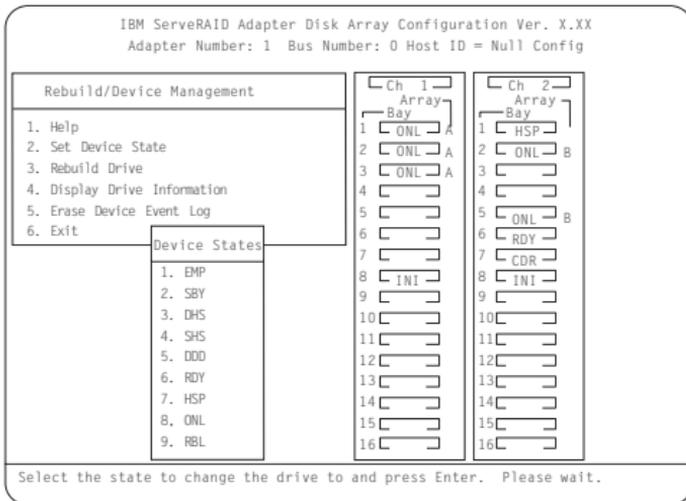
The Drive States pop-up window lists all hard disk drive states. (See “Physical Device States” on page 86 for more information.) The following table shows the current device states and the valid alternate device states that you can assign. For example, you can change the state of a standby hot-spare drive from SHS to HSP or DHS.
