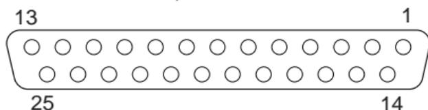
The following table shows the pin-number assignments for the parallel-port connector.
