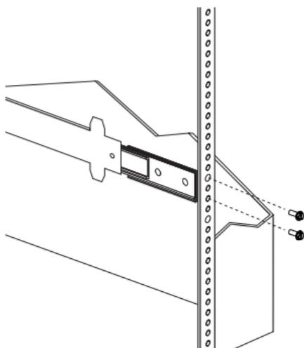
4. Attach the slide bracket assembly to the rear of the rack:
