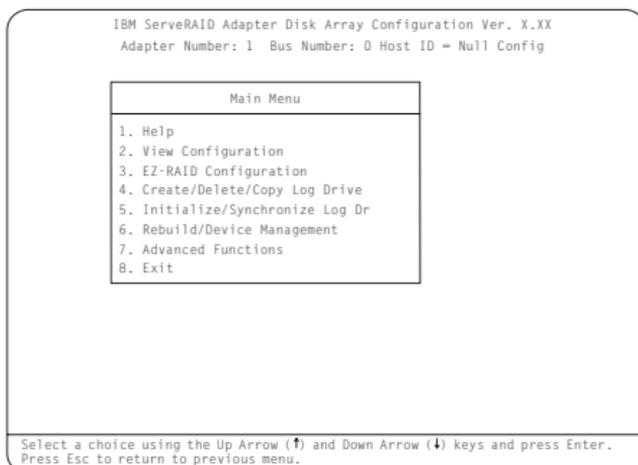
Type the highlighted number of the menu item, or use the Up Arrow (↑) or Down Arrow (↓) key to highlight your choice; then, press **Enter**. You can also press **Esc** to return to the previous menu, the previous work area of a screen, or to the beginning of the Main Menu.
