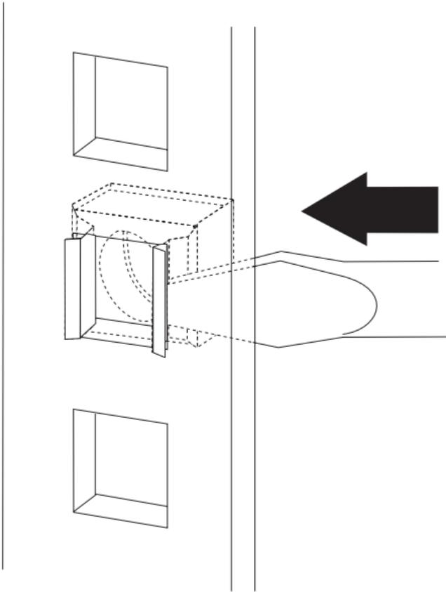
2. With the cage nut-clip compressed, push the cage nut-clip out of the square hole.
