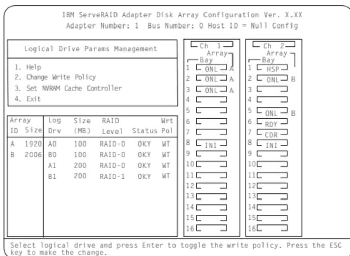
5. Locate the **Wrt Pol** field in the Logical Drive list. The write policy is shown as either write through (WT), which is the default setting, or write back (WB).
