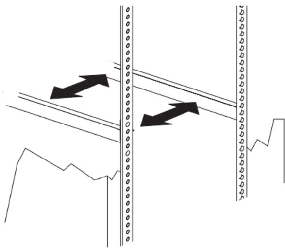
7. Tighten all screws to secure both slide-bracket assemblies. If you are using a torque screwdriver, use the following torque setting: 8–11 Nm (70.8–97.0 in/lbs).
