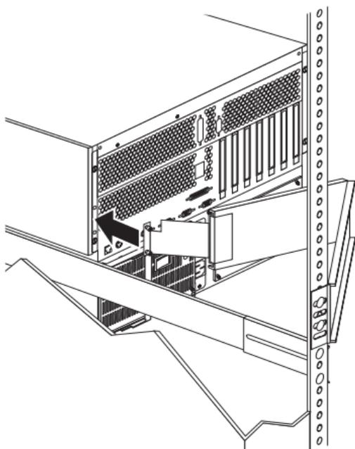
9. Attach the monitor, keyboard, and power cables to the corresponding connectors on the server. Refer to the rack documentation for instructions.
