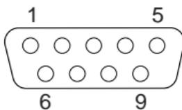
The following table shows the pin-number assignments for the serial-port connectors.
