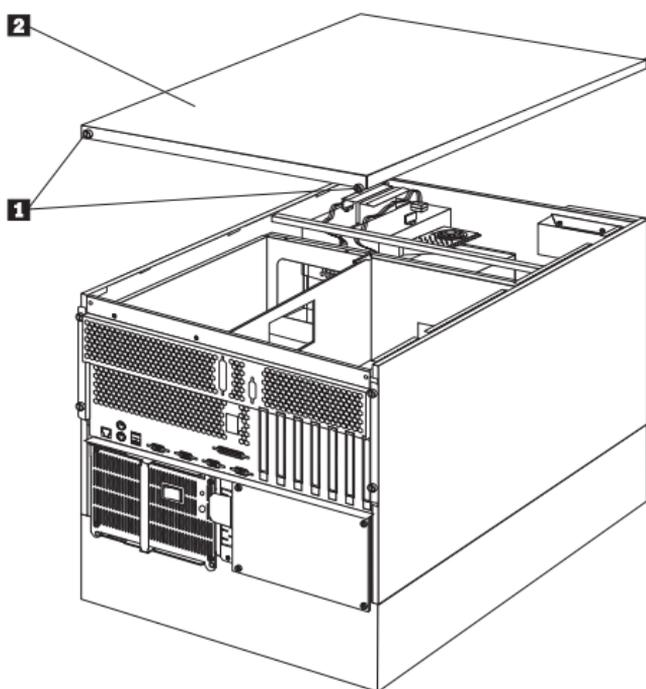
4. Tighten the two thumbscrews **1** on the back edge of the cover.
