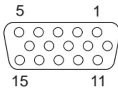
The following table shows the pin-number assignments for the video connector.
