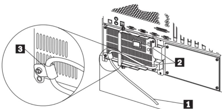
5. Plug the power cord into a properly grounded electrical outlet.
