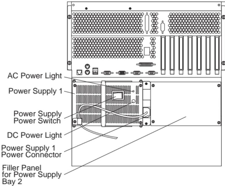
**Hot-Swap Power Supplies:** Your server comes with one hot-swap power supply installed. You can install a second hot-swap power supply to provide redundant power. You cannot hot swap a power supply if your server has only one power supply installed. (See “Hot-Swap Power Supply Installation” on page 181 for instructions.)
