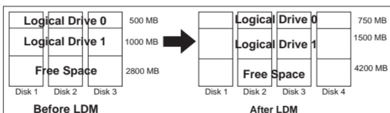
For example, an existing array uses three 2150 MB hard disk drives that are configured as two RAID level 5 logical drives (one 500 MB and one 1000 MB) and 2800 MB of free space. If you use the logical-drive migration procedure and add a 2150 MB hard disk drive to proportionally increase the size of the disk array, the end result will be two RAID level 5 logical drives (one 750 MB and one 1500 MB) and 4200 MB of free space.
