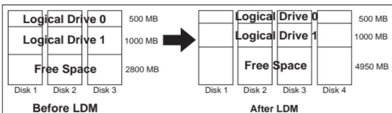
For example, an existing disk array uses three, 2150 MB hard disk drives that are configured as two
