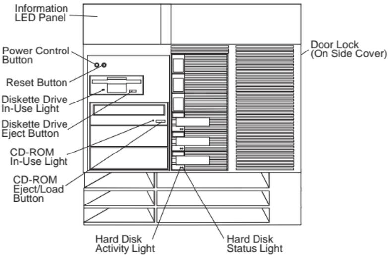
**Door Lock (Tower Model Only):** You can lock the door on your server to deter tampering with the internal components. This same lock also locks the top cover in place.
