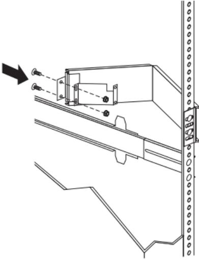
**Installing the Server in the Rack:** In this section, you will use eight screws (M4 by 8).
