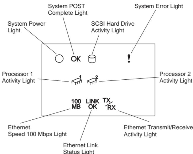
**System Power Light:** When this green light is lit, system power is present in the server. When this light flashes, the server is in standby mode (the system power supply is turned off and AC current is present). When this light is off, it indicates either power supply failure, an AC power failure, or a light failure.
