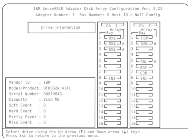
4. Use the Up Arrow (↑) or Down Arrow (↓) key to highlight the drives in the Array/Bay selection list. When you highlight the drive, the drive information appears as follows:
