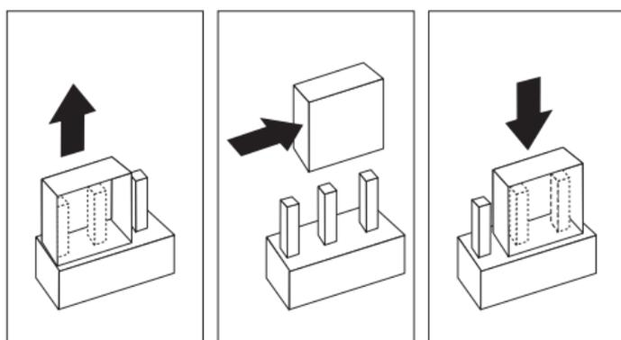
5. Slide the jumper fully onto these pins.
