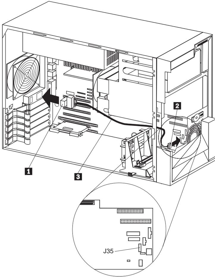
6. Connect the Advanced System Management Interconnect cable to the connector you just installed in the knockout on the back of the server.
