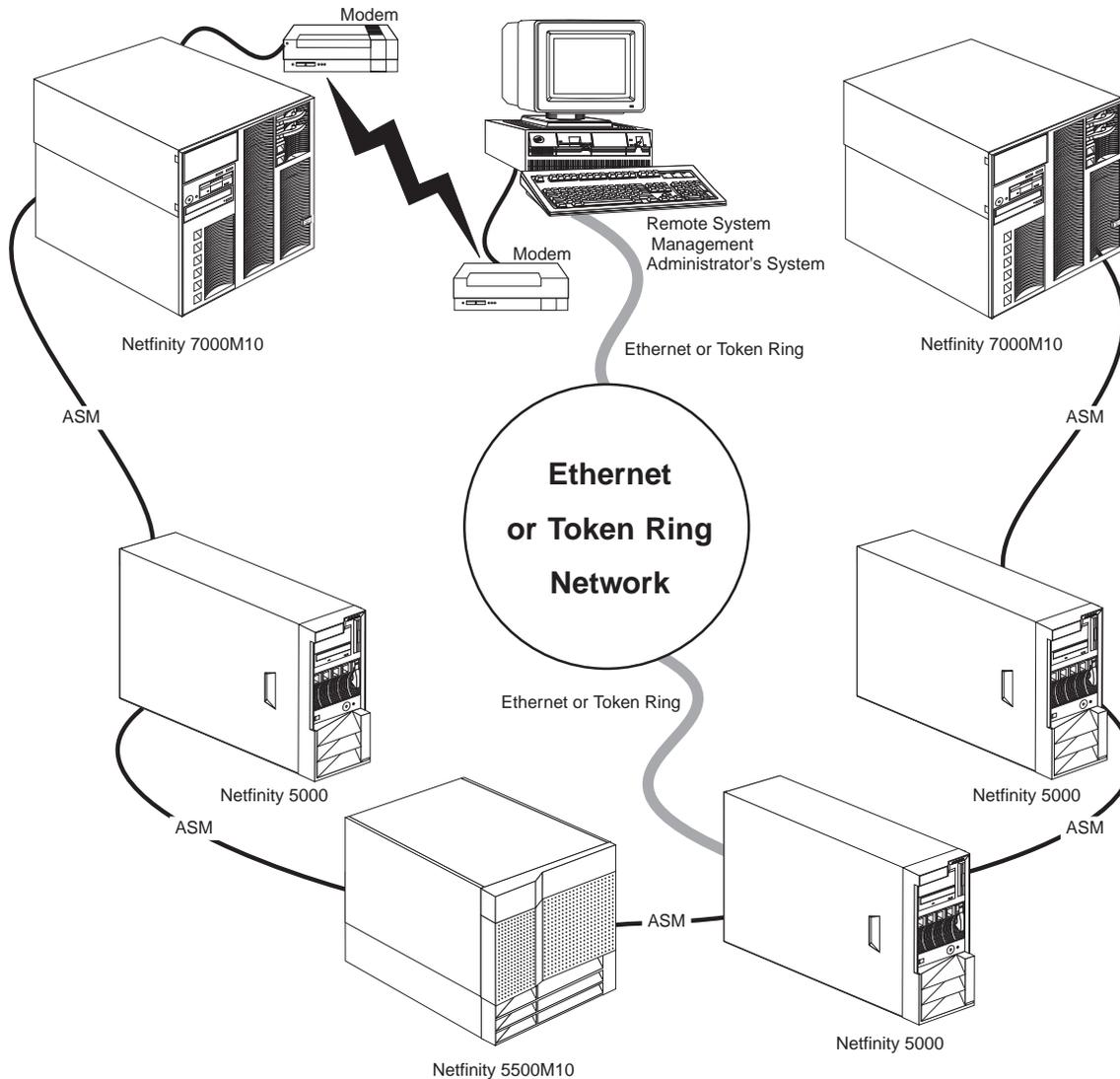
In this example, a modem has been connected to the Advanced System Management Processor in a Netfinity 5000. In this case, the Netfinity 5000 will use the modem to forward system management data generated by the other systems in the ASM Interconnect network bus to the remote system management administrator.
