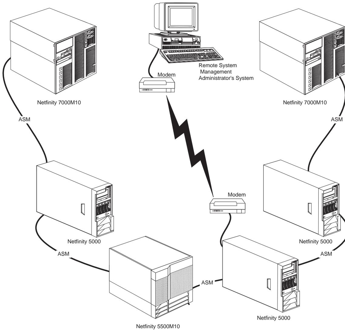
In this example, modems have been connected to the Advanced System Management PCI Adapter that is included with Netfinity 7000 M10 servers at each end of the ASM Interconnect network bus. Placing modems at opposite ends of the ASM Interconnect network bus ensures that if an ASM Interconnect connection in the bus fails all of the systems will still have access to a modem to forward system management data to the remote system administrator.
