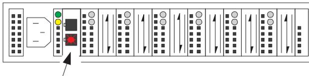
To verify the integrity of the fiber optic cable at the node end of a link, make sure the cable is attached to the GBIC at the hub and the hub is turned on. Dual SC fiber-optic cable connectors are keyed and will insert into a GBIC in one direction only. Place a mirror at the node end of the link. A low intensity red light is visible in the mirror reflection of one of the SC leads, as shown in the following illustration.
