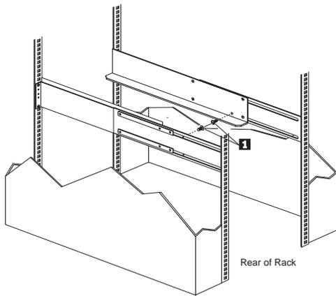
6. Remove the two small 6-32 screws **1** on the interior side of the rails. Save these screws to install the Expansion Unit
