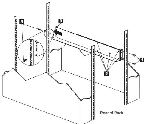
2. Loosen the five screws (four large screws and one small screw) **2** located on the interior of the rail
