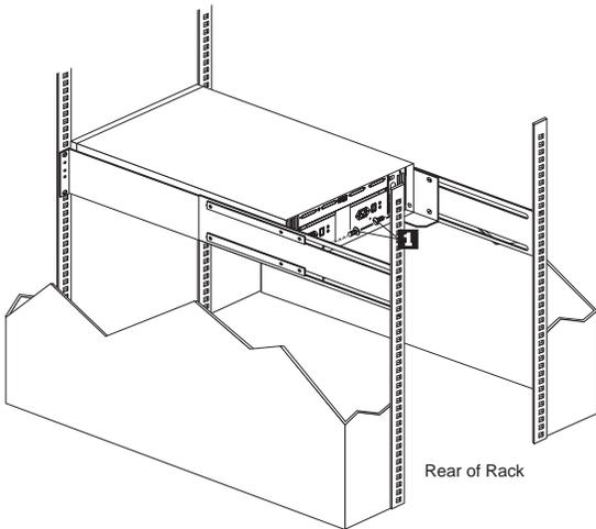
1. Remove screws **1** from assembly rails at rear.
