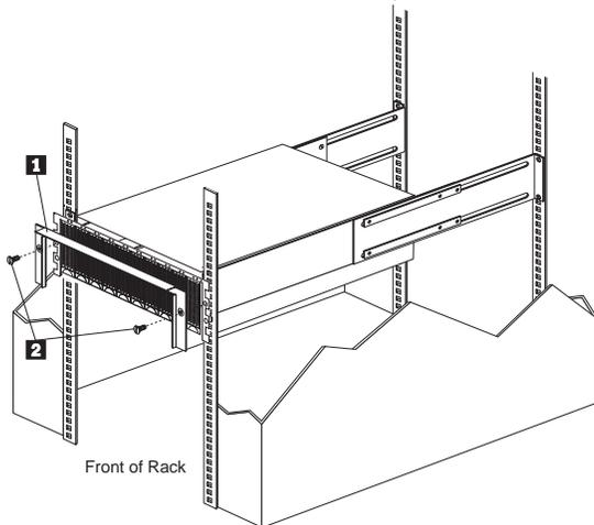
2. Remove screws **2** and remove bezel **1**.
