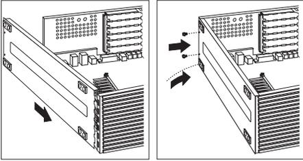
3. Align the holes and insert the two bottom screws.
