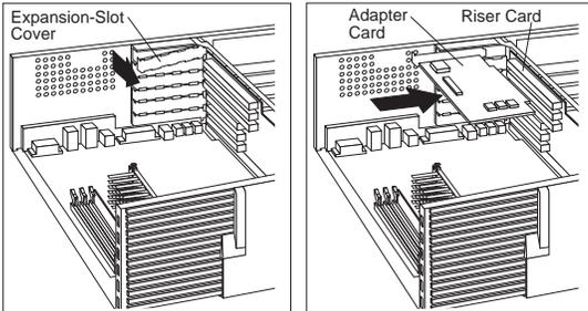
8. Install the bracket and the screw.
