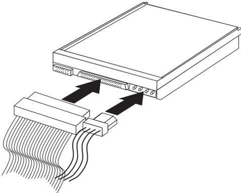
6. If you have installed a drive with removable media, you must remove the bay panel (bezel). If you have installed a drive with nonremovable media, you must install a bay panel (if it was not already installed).
