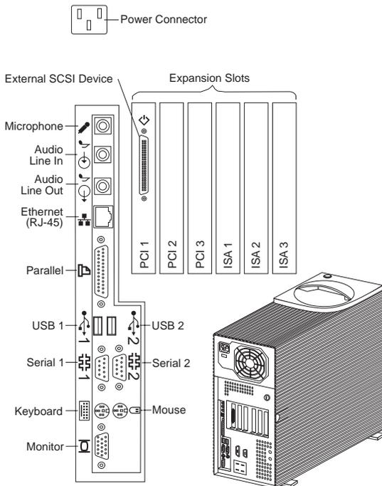
**Power Connector:** The server power cable connects here.
