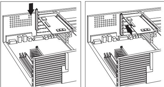
9. If you installed a network adapter that uses Wake on LAN or Alert on LAN, attach the cable from the riser card to the adapter. See "ISA and PCI adapters" on page 62 to locate the Wake on LAN or Alert on LAN connector. If you installed a modem and want to use Modem Wakeup, see "ISA and PCI adapters" on page 62 to locate the Modem Wakeup connector on the riser card.
