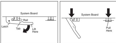
7. Using the tab, slide the system board out and set it aside.
