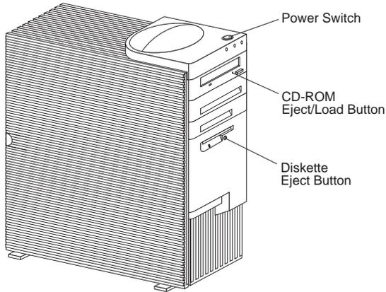
**Power Switch:** Press this switch to turn the server on or off.
