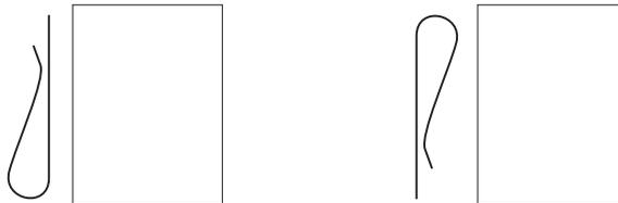
The open end of the wavy marks indicates the direction the open end of the clip must face. (One clip must face the open side of the server; the other clip must face the system board.)
