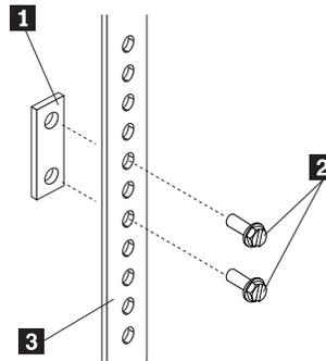
4. Attach nut bars to the other three corners of the U-unit in the same way.
