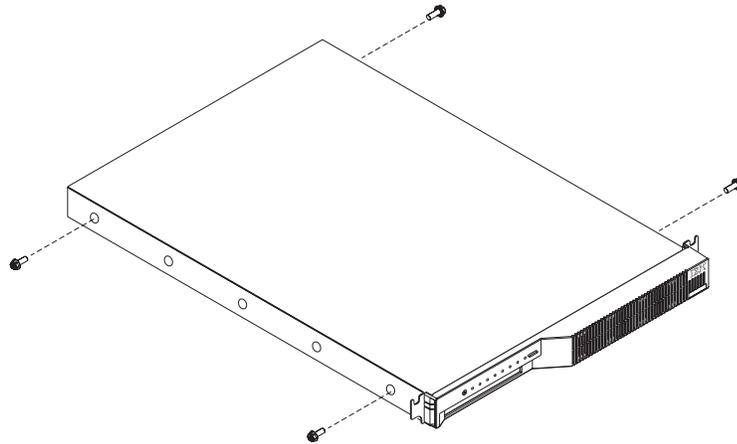
3. Attach the inner slide section of each slide rail assembly to the side of the server.
