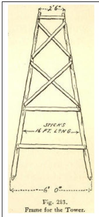
Fig. 283. Frame for the Tower.
