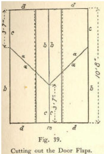
Fig. 39. Cutting out the Door Flaps.
