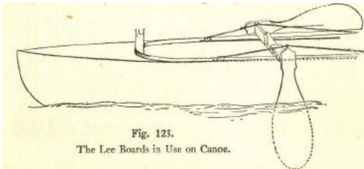
Fig. 123. The Lee Boards in Use on Canoe.
