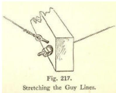
Fig. 217. Stretching the Guy Lines.
