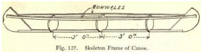
Fig. 127. Skeleton Frame of Canoe.
