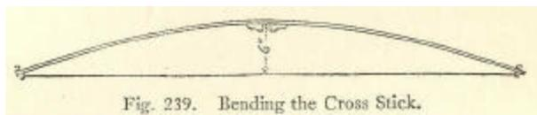
Fig. 239. Bending the Cross Stick.
