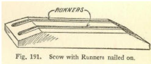
Fig. 191. Scow with Runners nailed on.
