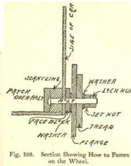
Fig. 300. Section Showing How to Fasten on the Wheel.
