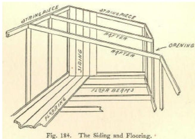
Fig. 184. The Siding and Flooring.
