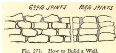
Fig. 273. How to Build a Wall.
