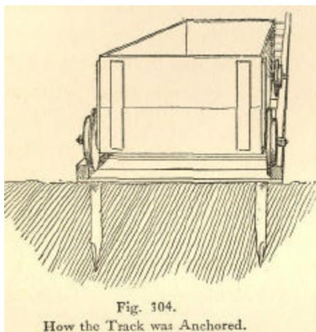
Fig. 304. How the Track was Anchored.
