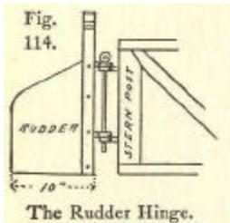
Fig. 114. The Rudder Hinge.
