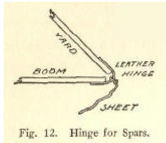
Fig. 12. Hinge for Spars.
