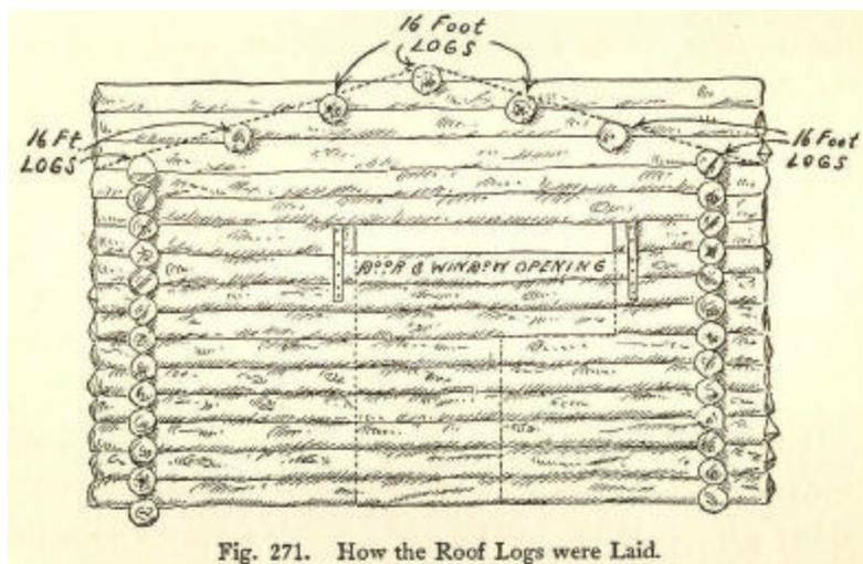
Fig. 271. How the Roof Logs were Laid.
