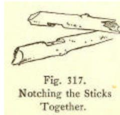
Fig. 317. Notching the Sticks Together.
