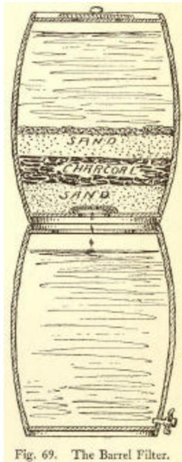
Fig. 69. The Barrel Filter.
