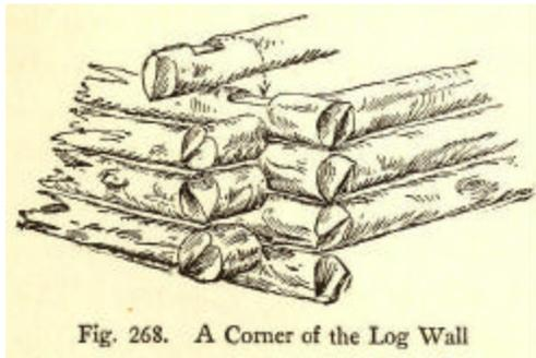
Fig. 268. A Corner of the Log Wall.
