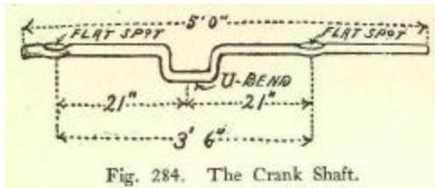
Fig. 284. The Crank Shaft.
