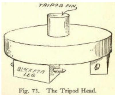
Fig. 73. The Tripod Head.
