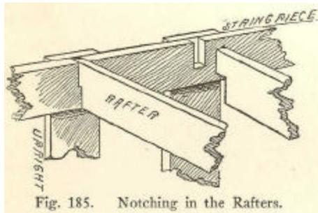
Fig. 185. Notching in the Rafters.
