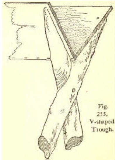
Fig. 253. V Shaped Trough.
