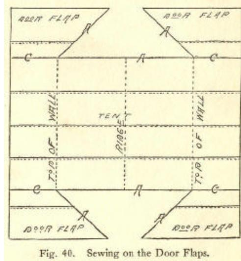
Fig. 40. Sewing on the Door Flaps.
