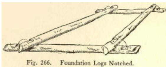
Fig. 266. Foundation Logs Notched.
