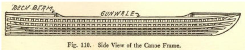
Fig. 110. Side View of the Canoe Frame.
