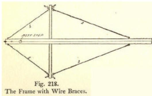
Fig. 218. The Frame with Wire Braces.
