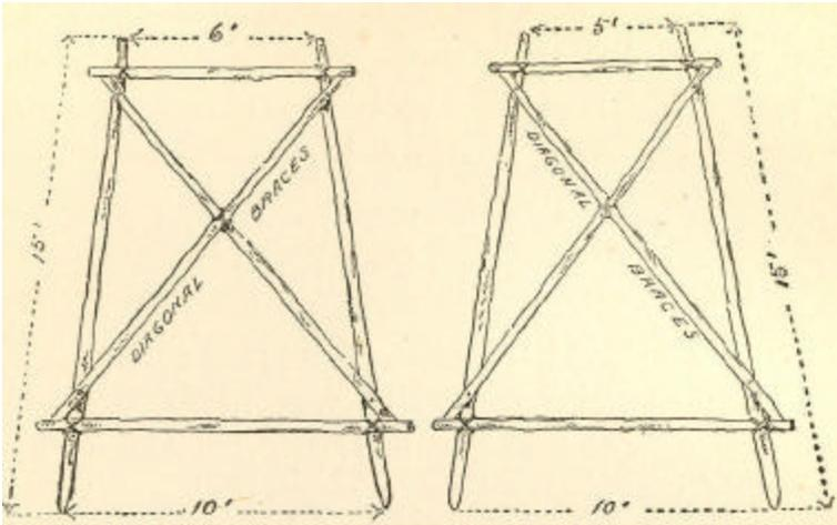
Figs. 91 and 92. Frames for the Spar Bridge.
