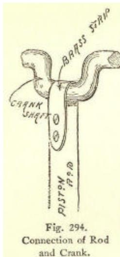
Fig. 294. Connection of Rod and Crank.
