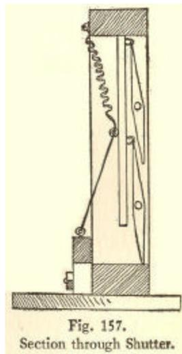
Fig. 157. Section through Shutter.
