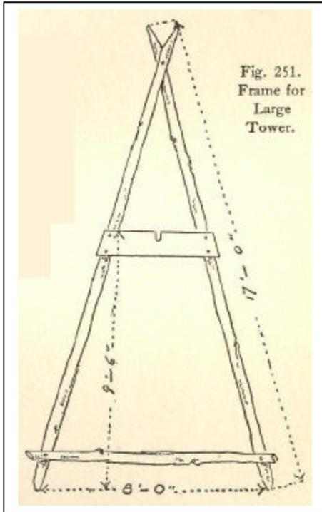
flattened at their upper ends and nailed together, with the ends projecting about a foot, as shown in Fig. 251. At the bottom these poles were spaced 8 feet apart by a cross bar, and about 9-1/2 feet from the bottom a pair of boards were nailed to opposite sides of the pole to serve as supports for the axle of the water wheel. Another pair of 17-foot poles was now similarly fastened together and then the two pairs were spaced about 12 feet apart and connected at the top and bottom with boards.
