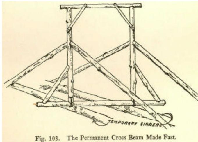
Fig. 103. The Permanent Cross Beam Made Fast.
