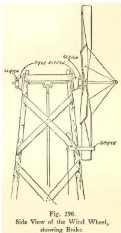
Fig. 290. Side View of the Wind Wheel, showing Brake.
