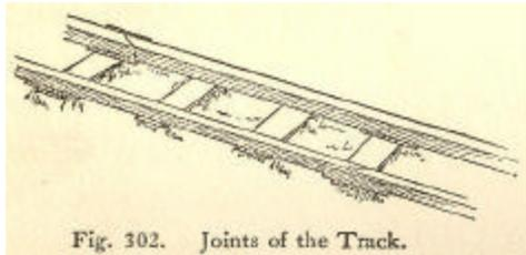
Fig. 302. Joints of the Track.
