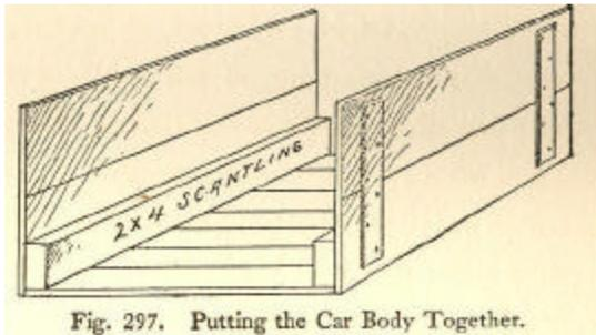
Fig. 297. Putting the Car Body Together.
