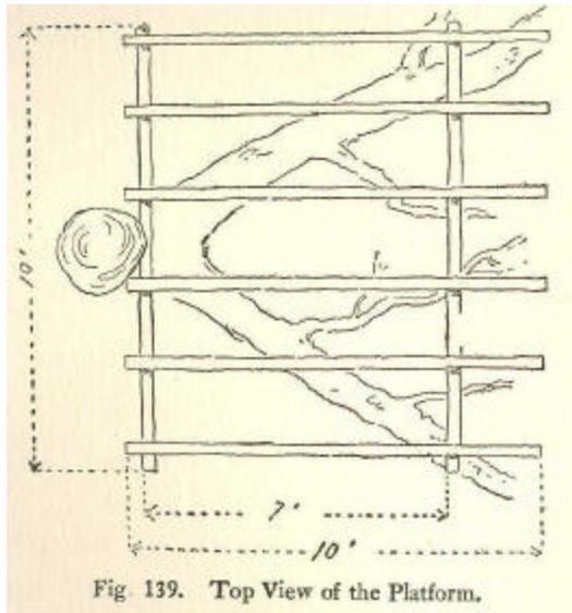
Fig. 139. Top View of the Platform.
