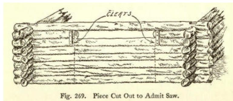
Fig. 269. Piece Cut Out to Admit Saw.
