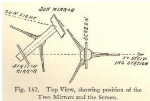
Fig. 162. Top View, showing position of the Two Mirrors and the Screen.
