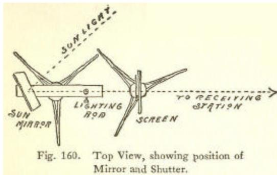
Fig. 160. Top View, showing position of Mirror and Shutter.
