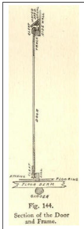
Fig. 144. Section of the Door and Frame.
