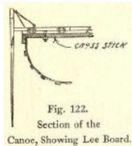
Fig. 122. Section of the Canoe, Showing Lee Board.
