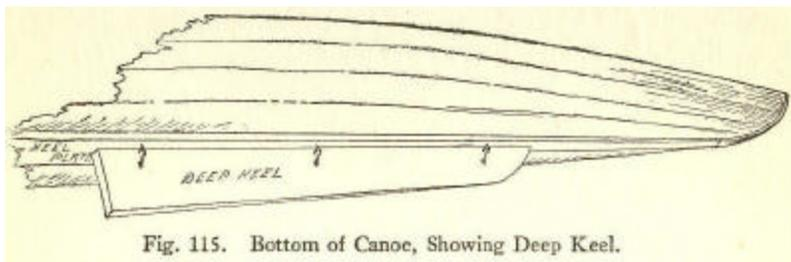
Fig. 115. Bottom of Canoe, Showing Deep Keel.
