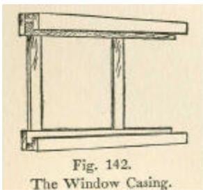
Fig. 142. The Window Casing.
