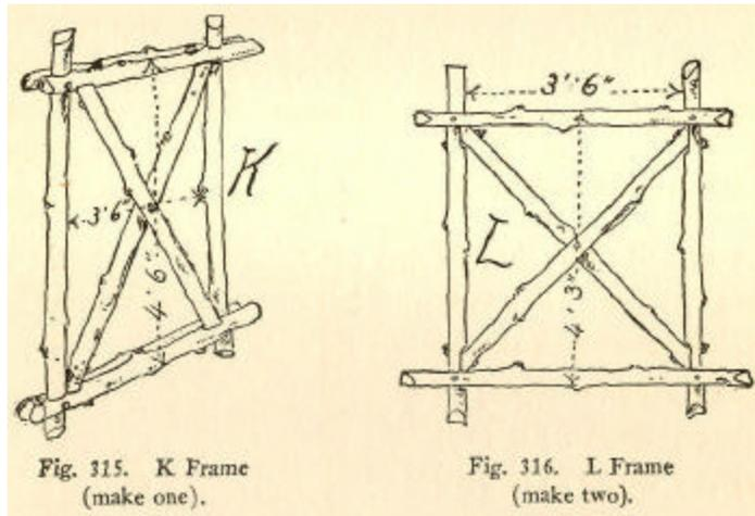
Fig. 315. K Frame (make one).      Fig. 316. L Frame (make two).
