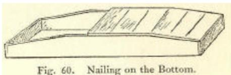
Fig. 60. Nailing on the Bottom.
