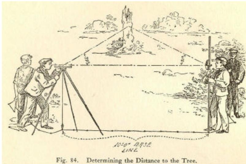
Fig. 84. Determining the Distance to the Tree.
