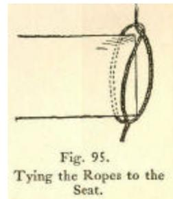
Fig. 95. Tying the Ropes to the Seat.
