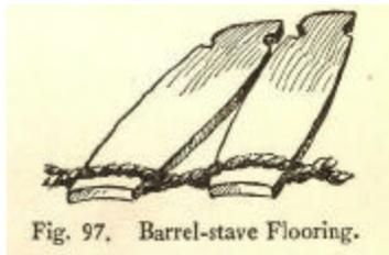
Fig. 97. Barrel-stave Flooring.
