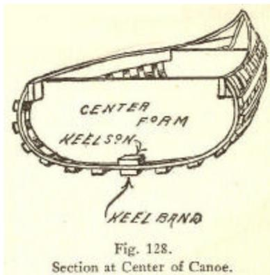
Fig. 128. Section at Center of Canoe.
