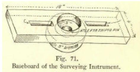
Fig. 71. Baseboard of the Surveying Instrument.
