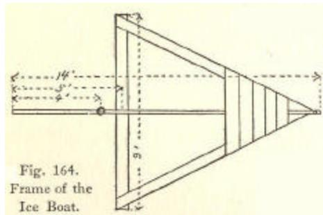
Fig. 164. Frame of the Ice Boat.
