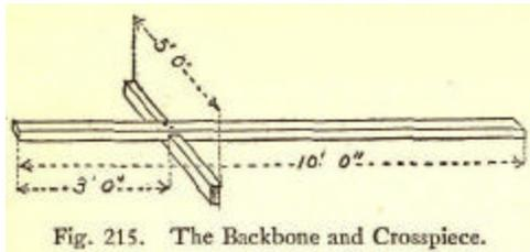
Fig. 215. The Backbone and Crosspiece.
