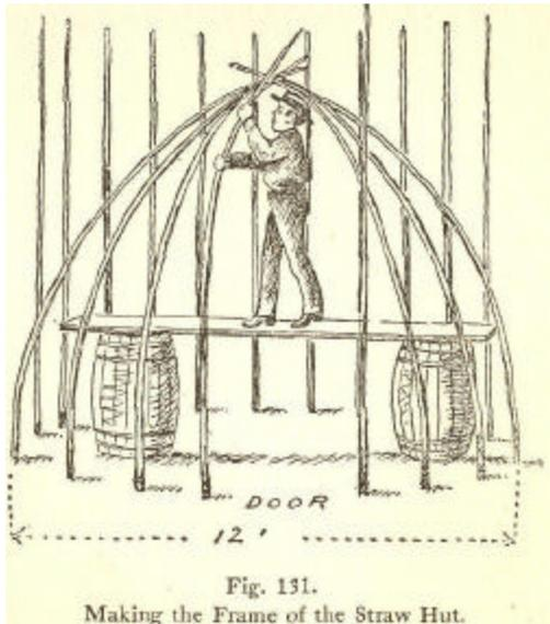
Fig. 131. Making the Frame of the Straw Hut.
