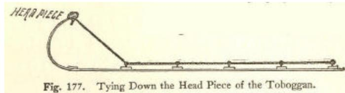
Fig. 177. Tying Down the Head Piece of the Toboggan.
