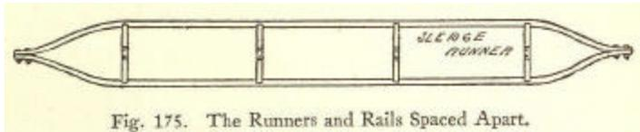
Fig. 175. The Runners and Rails Spaced Apart.
