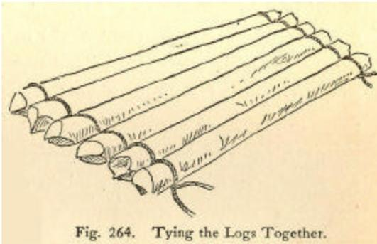
Fig. 264. Tying the Logs Together.
