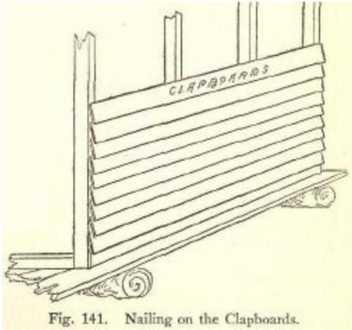
Fig. 141. Nailing on the Clapboards.
