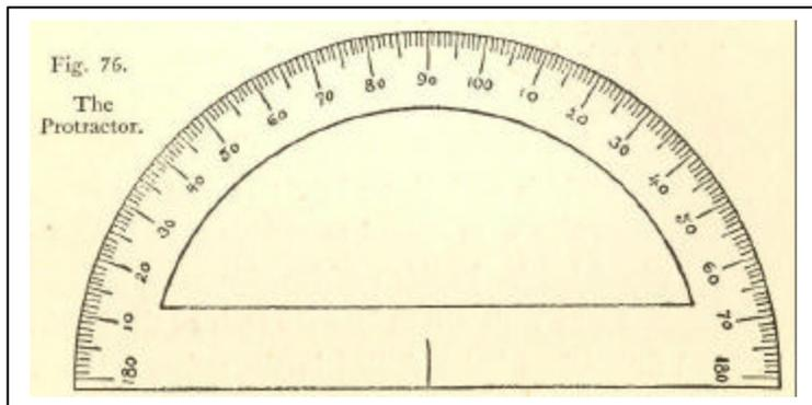
Fig. 76. The protractor.
