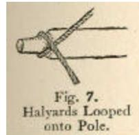
Fig. 7. Halyards Looped onto Pole.
